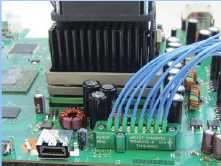
Fig-1 Terminate-R mounted to PCB
