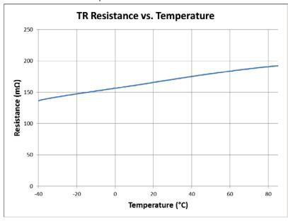
Resistance Tolerance:  $\pm 17 \text{ m}\Omega$  at (21.1 °C)
