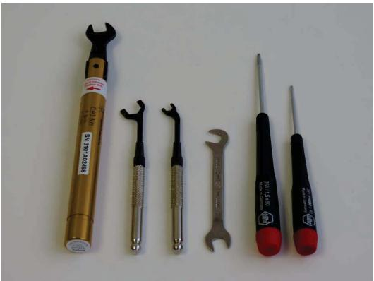
Figure 10: Recommended Permissible Hardware Instruments
