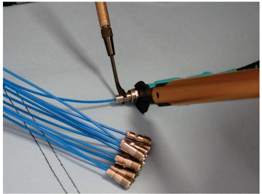
Figure 11: Connection Torque Procedure
