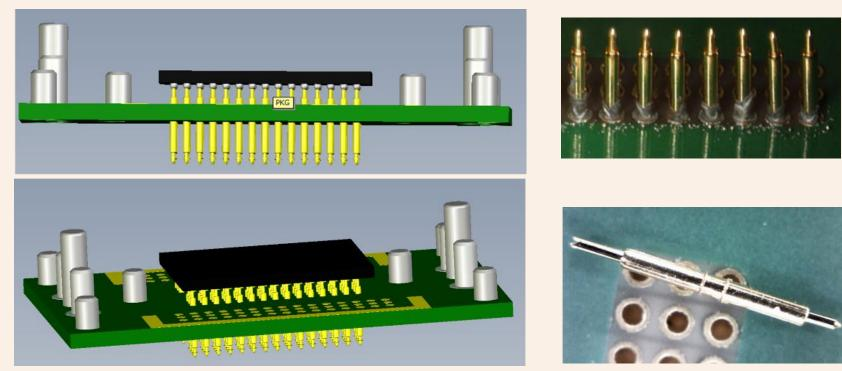
Example PKG: BGA (DDR3 memory) Pitch: 0.8mm Pin count: 96 pin
