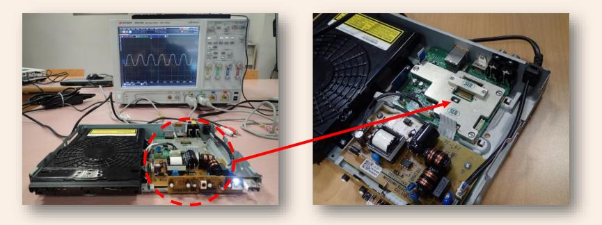
Signal probe socket is on a board of DVD player and connected to the oscilloscope.
