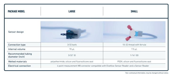
SENSOR SIZE (length x width x height): LARGE: 29 x 13 x 27 mm SMALL: 40 x 33 x 19 mm AMPLIFICATION MODULE SIZE: 52 x 24 x 24 mm
